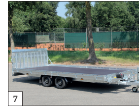
7 Standard: tyres 195/50 R13 C with black rims for the models in 450 and 505 cm with parabolic leaf spring axles.
