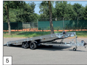
5 Standard: Parabolic leaf spring axles incl. shock absorbers for the models in 450 and 505 cm length (lowered floor height with parabolic axles!).
