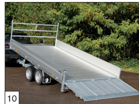
10 Option: aluminium dropsides 300mm and a ladderrack in front. (a ladderrack is only possible in combination with dropsides).
