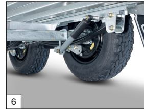
6 Parabolic leaf spring axles incl. shock absorbers (parabolic axles not possible for models in 405 cm).
