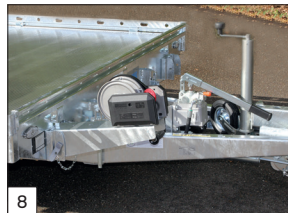
8 Standard: a multi-adjustable winch with support mounted in front.
