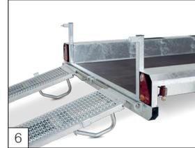
**Option:** 2 steel galvanised loading skids with a length of 1500 mm, hinged at the back.
