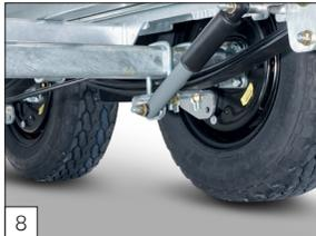
**Option:** parabolic suspension including shock absorbers.
