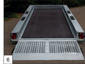
6 Standard: a drive on ramp consists of an open anti-slip grating profile the ramp is full-immersion galvanized and with springs.
