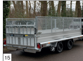
15 Option: wire rack extension 75 cm high including walls 30 cm high. Total 105 cm high, removable.
