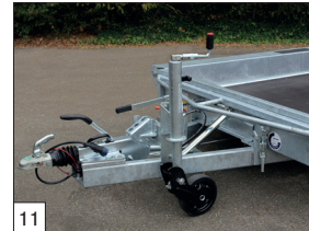
11 Standard: an extra reinforced tilting jockey.
