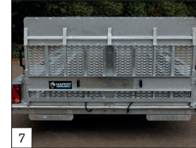
7 Standard: a drive on ramp in one piece 1200 mm high, including 2 removable corner pillars and adjustable heavy duty fasteners.
