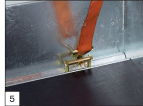
5 Standard: 1000 daN (KG) each fixing point.
