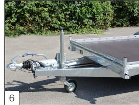
**Standard:** the braked models have been provided with a screwed on V-drawbar and a foldable jockey wheel. The unbraked models have a screwed-on tube drawbar and a light-weight jockey wheel.
