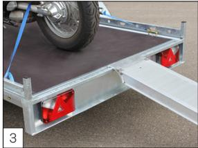
**Standard:** U profile at the rear for the mounting of one or more loading skids.
