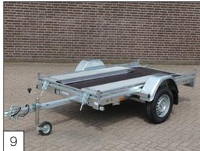
**Standard:** Indigo L-1 is available as an unbraked version in 750 kg or a braked version in 1350, 1500 or 1800 kg.
