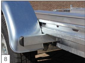
**Standard:** 4 mudguard supports to mount the mudguards.
