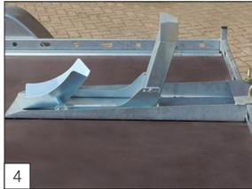
**Standard:** fixed Combi Protect Rail (with a height of 80 mm) on the front and sides. The adjustable motorcycle support is an option.
